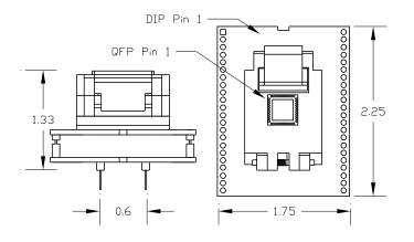
**Note:** The signal positions on the QFP device are rotated 180° from their respective DIP positions. To use this adapter insert the QFP device in the socket with pin 1 in the lower right-hand corner (see picture above).
